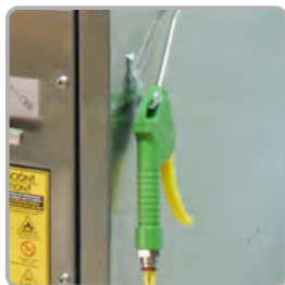
Blowgun for drying the gun interior areas.
