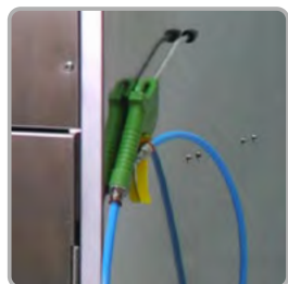
Gun with coupling for cleaning interior areas
