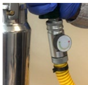
Product regulator by roulette with flow indicator
